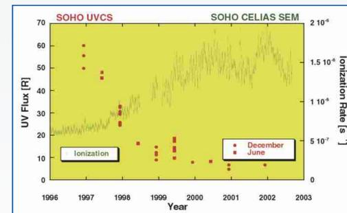
Intensity of the He 1584 Å glow of the focusing cone at 0.1 - 0.2 AU distance from the sun as taken with SOHO UVCS during June and December, 1996 through 2002. It is apparent that the He cone is strongly depleted as the ionization rate increases towards maximum solar activity.
