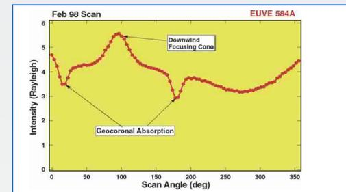
The flux increase in the center represents the cone. The second increase reflects the Earth's exospheric glow. The two dips are caused by resonant absorption of the He line by the exosphere in the directions where the velocity of the interstellar gas relative to the Earth is zero. The exact location of these features are used to deduce the He flow velocity.
